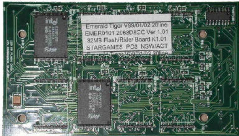
The Flash Rider Board is used for the storage of game media for the machine and can be interchanged with other approved game media modules to change the game characteristics. The board is fitted into the two parallel sockets located on the tail of the memory board. Although the module is designed so that it can be fitted in only one way, care should be taken to ensure that the pins within the connectors are not damaged when fitting this unit to the memory board.
