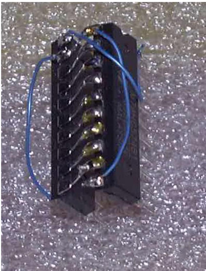
U43 is the socket for the Bipolar PROM which is IGT's "CAPROM". This is a small PROM which contains the color pallet for the Graphics. You would need to locate the proper CAPROM that goes with the 4 CG Graphics chips installed on your board.
