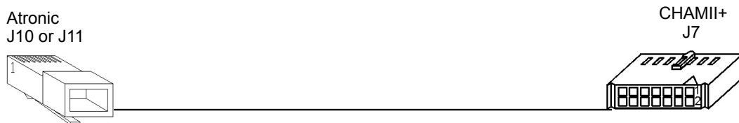
Figure A.1 Atronic to CHAMII + harness 311-205-05
