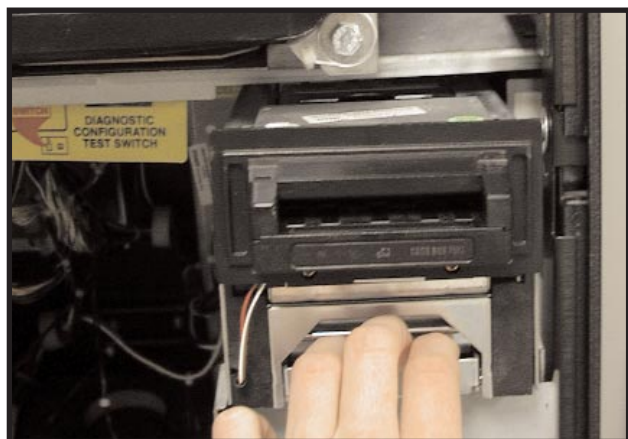
Image 15. Removing the Bill Validator.
