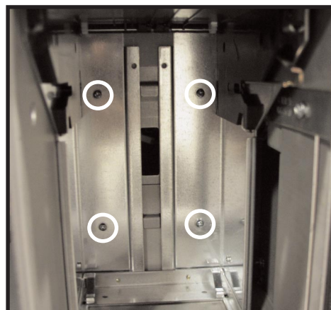
Image 16. Four Phillips screws to remove.
