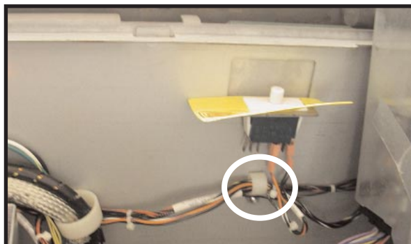
Image 36. Cable clamp for power cable, located below the Monitor shelf (550).
