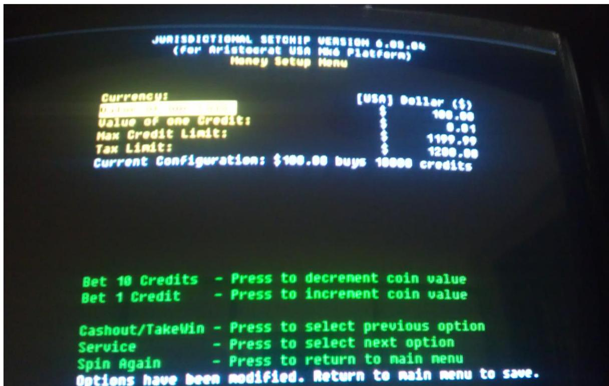
Once your screen looks exactly like mine below (be sure the version is 06.03.04) ,Scroll to "Save All Options" and select. After it's saved, power down the machine and remove the set chip extender board.
