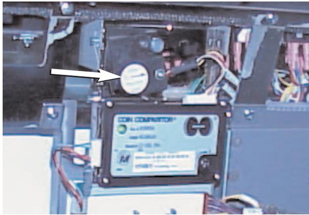
1. If the game has a Coin Mechanisms Micro Comparator 40 (MC-40) or the Coin Comparator 16 (CC-16), install a sample coin of the proper denomination into the Comparator. IDX Coin Xeptors and the Condor validators will already be calibrated in the factory to use the Hopper's denomination. NRI coin validators are preprogrammed. To program, see the Periodic Service Chapter.
