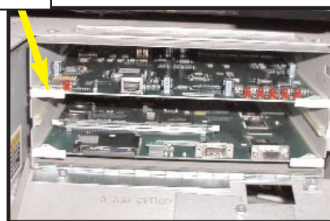
Image 4a (left) and 4b . CPU and I/O boards installed, 55x (left), and 36x.
