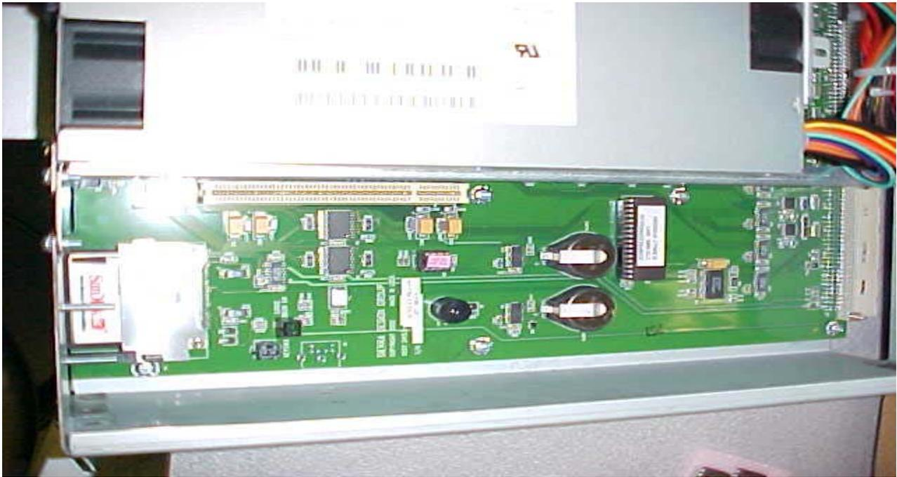
Install the Cables CBL-20522-0001 into the three-prong connector at the upper left of the backplane of the Alpha Machine.
