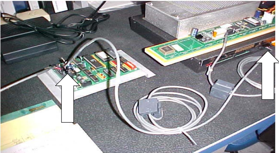
From J5 on the Super Controller run cable CBL-20524-0001 to J1 on the CAM III which is connected to the back of the 12 Cell Mini Photon.
