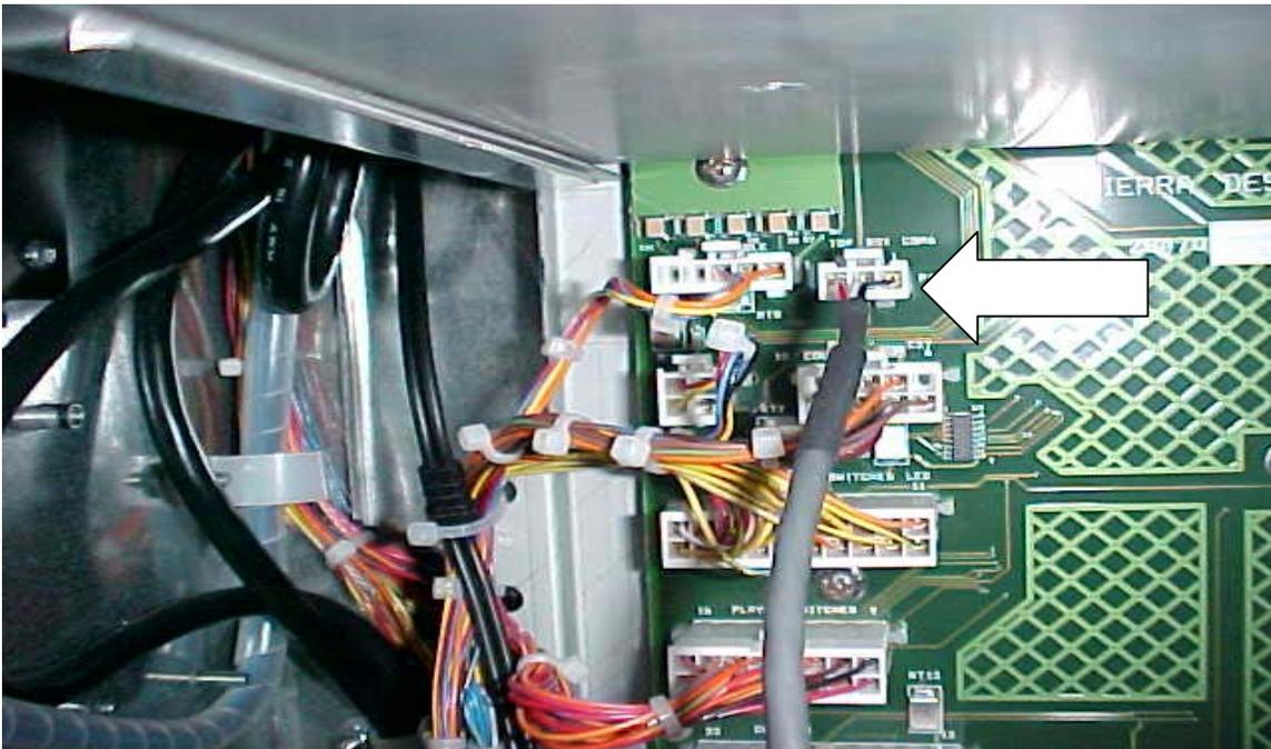
This cable will connect to J2 on the SIB board AS-02982-0064. The SIB board has a power supply that also plugs into the board in the round jack on the end of the board. This supply has a 12V and 1.5A output. This is the smaller supply in the kit.
