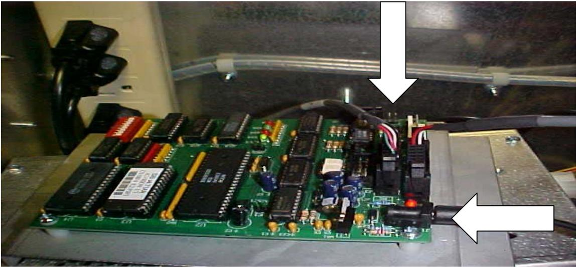
Use cable CBL-20423-0001 to connect J3 of the SIB board to J3 of the Super Controller.
