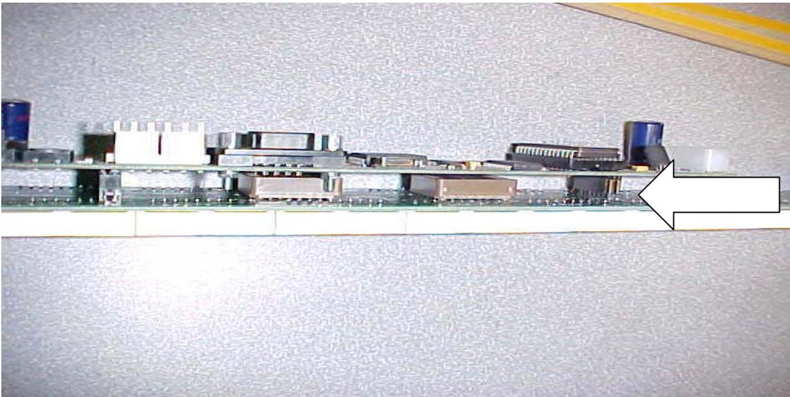
The Super Controller also has a power supply that is connected to it at the jack on the right end in the front on the unit. This power supply has an output of 12V and 2.5A. This is the larger supply in the kit and has a higher current output than the other supply included in the kit. All the power supplies should be connected to the power strip.
