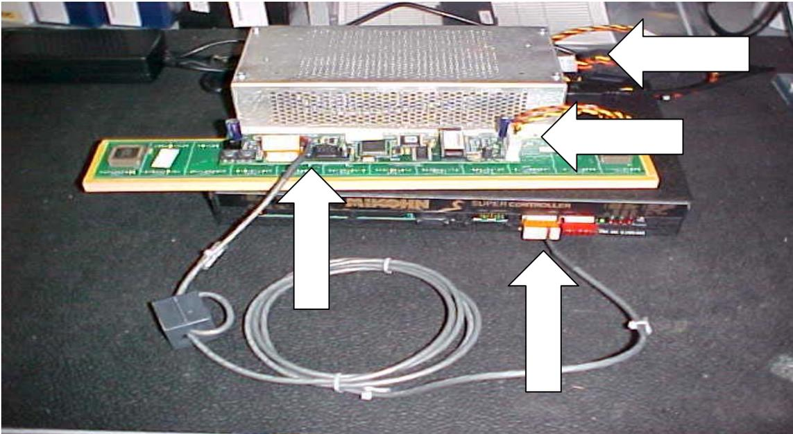
The CAM III and 12 Cell Mini Photon has a power supply from K-00621-9001 that also needs connected. Connect the power cord to a Splitter box and plug it in the end at the power connection. Install the multi-colored cable from the kit into the jack on the end of the power unit and plug the smaller end of the cable into the back of the CAM III. Make sure that the CAM III is connected to the 12 Cell Mini Photon properly. The connectors used here can be plugged incorrectly.
