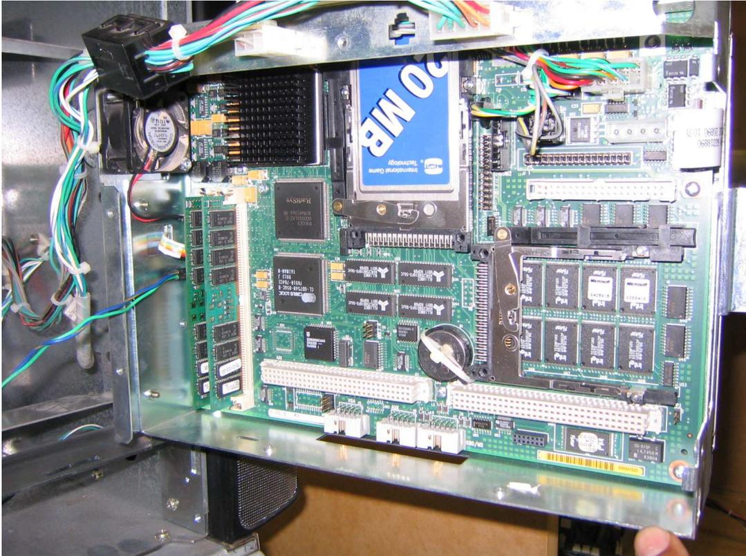
3. Remove the PCMCIA in the top slot of the LCD.
