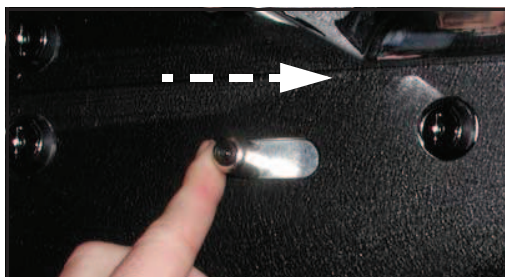
Figure 2-92 Releasing the Participation Cap Door.
