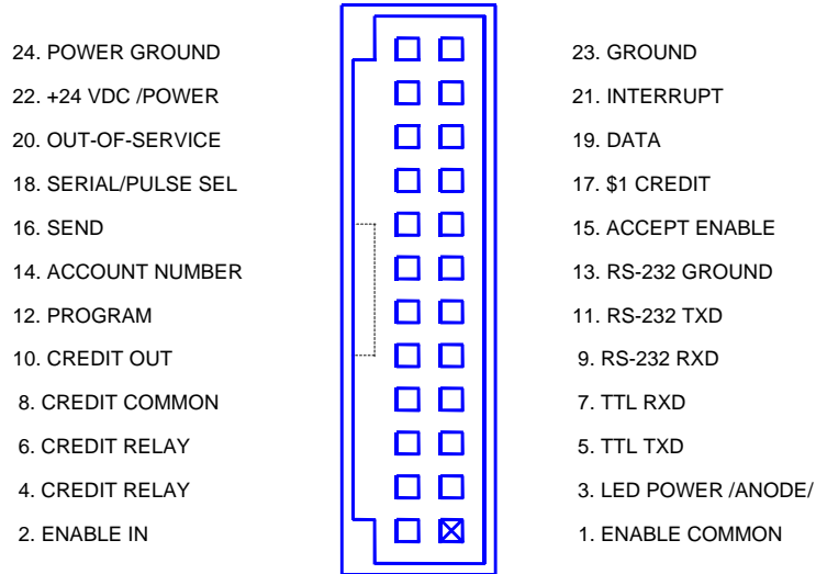
Figure 6. Currency Validator 24-Pin Main Connector
