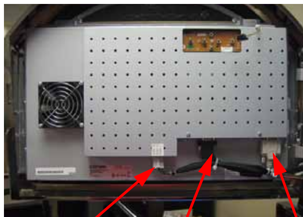
DC Monitor connector, Video Cable, and Touch Screen Cable.
