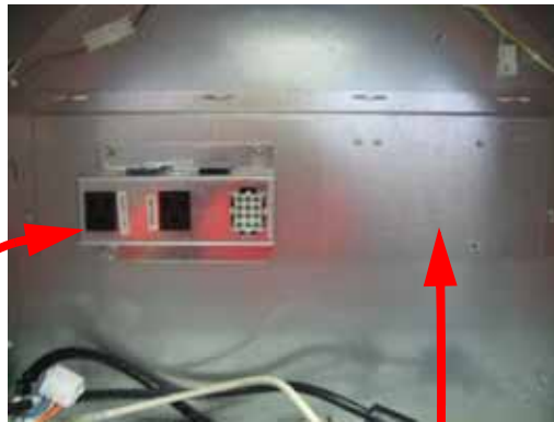
Convenience Outlet (201339) and Bottom Component Mounting Panel (202004).
