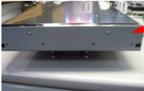
Left LCD Monitor Bracket (206138).
