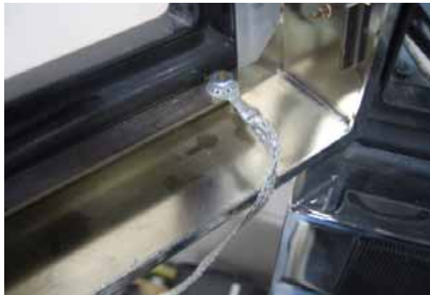
Ground Strap (200003-00006) secured to Top Door.
