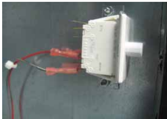
Door Push Switch and bracket.
