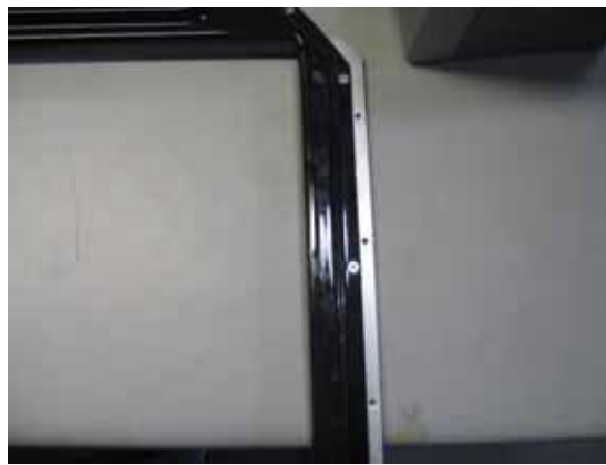
Right Bezel Bracket (200512) (third hole and screw not shown).
