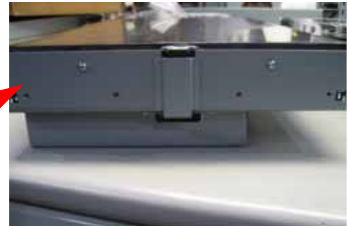
Right LCD Monitor Bracket (206137).
