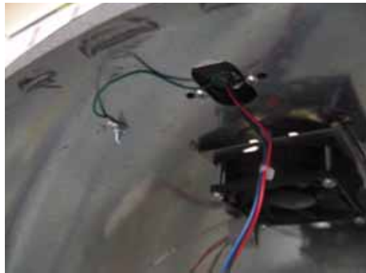
Ground wire connected to standoff.
