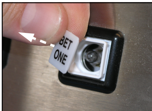
Figure 7 Removing the insert from the button.
