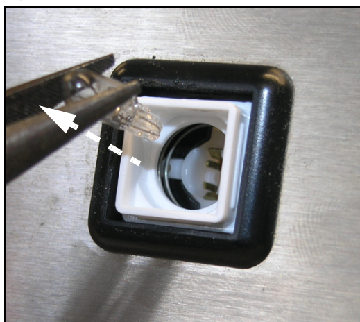
Figure 9 Pulling the lamp from the socket.
