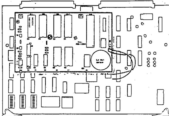
Controller Board with MCU module
